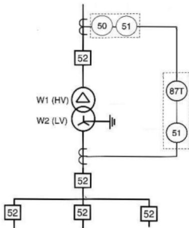
Two-winding transformer protection
